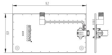
The testboard is designed for evaluation purposes for the Picea 2.4 GHz. The card has the same size as a typical PCMCIA card. The board is fitted with an SMA connector.
