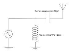
The testboard is matched with above specified components.
