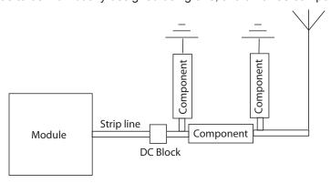
The schematic picture describes the radio module and the matching network. The matching network shall be designed as a PI net. The antenna acts as an active part of the device, the number and value of matching components will be unique for your application.
